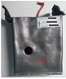
Single layer of poorly wrapped lead - significant leakage radiation detectable from all direction
