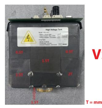
Multiple layers of lead, carefully wrapped especially around the X-ray generator tube - radiation only detectable from the X-ray focal spot
